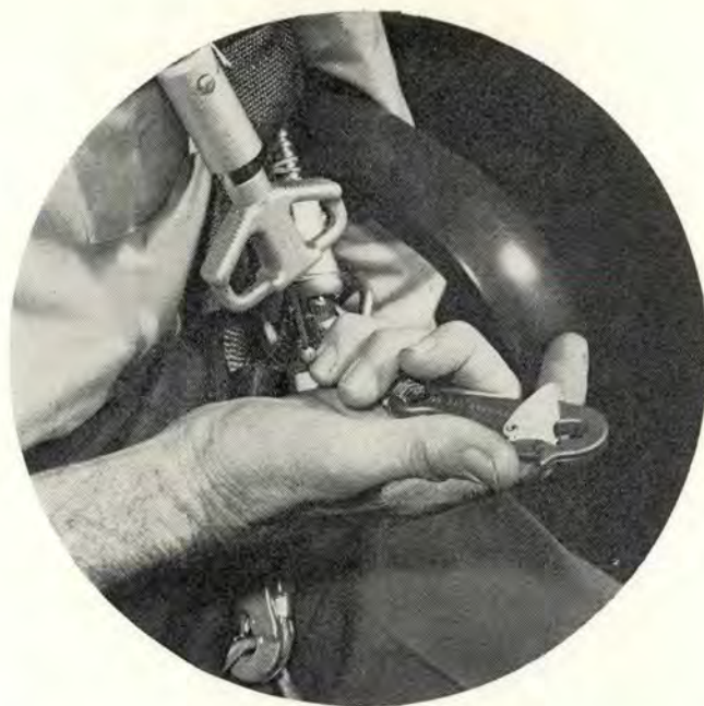
Grasp the fabric webbing of the lanyard immediately below the lanyard hook with the little finger and ring finger. The nose of hook is pointing at the thumb, the middle and index fingers are cradling the upper half of the hook, and the thumb is free and open.
